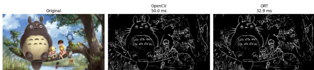
Comparison between OpenCV and ONNX runtime time execution performance on Sobel Edge Detector on an CPU execution provider (ORT : ONNX Runtime)
